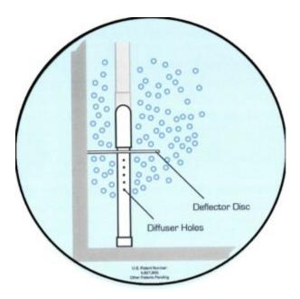
With the Aqua Aire<sup>®</sup> Deflector/Diffuser, air bubbles are dispersed in a wide area as they bounce off of the Deflector Disc on their way to the surface.
